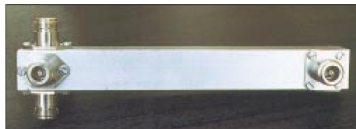
Figure 8: Self-built quadruple distributor for the 70 cm band
