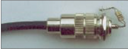
Figure 15: Home-brew 50 Ω terminating resistor for measuring the matching elements
