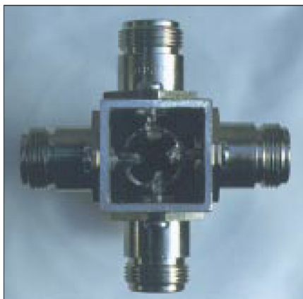
Figure 9: View into a quadruple distributor
