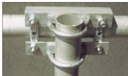
Figure 17: Mechanical realisation of the connection points for an Hshaped cross with aluminium brackets Photos: DK7ZB
